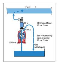
The auto air vent valve bleeds gas and liquid out of the pump chamber. However, pump output is maintained due to the feedback control from the flow sensor.
