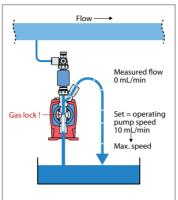
When a large volume of gas enters into the pump chamber, pump output will go to "zero" until the gas bleeds out. The feedback control increases pump speed, reducing the bleed time and quickly repriming the pump.
