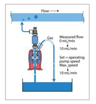
After the gas has been purged, the EFS sensor will begin to measure flow. Feedback from the sensor controls the pump, slowing it back down so the flow rate meets the set value.
