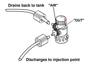
Figure 6 Air Vent Valve Tubing
