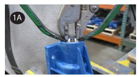
2 Plastic Air Valve - Remove and replace o-rings. Insert cap (item 6) push down until groove for the retaining ring is visible. Make sure to lubricate the o-rings prior to inserting into the valve body with a compatible lubricant.
