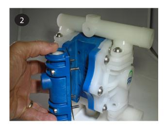
Place the new gasket (item 8) on the air valve (item 2) and ensure the slots in the gasket align with the slots in the air valve and valve plate (item 7).
