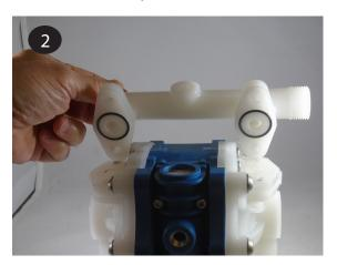
Repeat the above steps for the suction manifold (item12). The seat o-rings, valve seats and valve balls (items 13, 14, & 15) are located in the liquid chambers (item 18).
