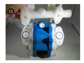
3 Stand the pump upright onto the suction manifold feet (item 12). Place the valve balls (item 15), valve seats (item 14), and seat o-rings (item 13) into the discharge manifold (item 16) in the same order as the suction side was done in step 11. Place the discharge manifold atop the pump, tighten, and torque the discharge manifold bolts (item 11) in an "X" pattern. Torque to 50 in-lbs (5.6 N-m).
