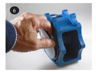
The remaining diaphragm (item 20) and plates (items 19 & 23) may be removed from the shaft (item 27) by hand or by placing the shaft in a vise fitted with soft jaws. Use a 6-sided 5/8" wrench to remove the remaining diaphragm and plates. Soft jaws are required to prevent damage to the shaft. A damaged shaft with result in accelerated o-ring wear. Jaws can be fitted with wood, plastic, rubber, or other soft material to prevent shaft damage.
