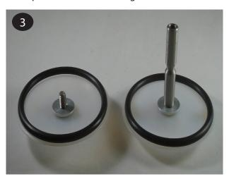
4 The shaft (item 27) and shaft bushing assembly (items 24. 25 & 26) should retain the lubricant that was factory applied. If they appear dry, apply a light coat of lithium thickened grease. Avoid over lubrication as it can cause decreased performance of the air distribution system.
