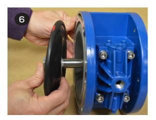
To remove the remaining diaphragm(s) (items 20/21) and plates (items 18 & 22) from the shaft (item 27), place the shaft in a vise fitted with soft jaws. Using a 6-sided 20mm wrench, remove the remaining diaphragm(s) and plates. Soft jaws are required to prevent damaging the shaft. A damaged shaft will result in accelerated o-ring wear. Jaws can be fitted with wood, plastic, rubber, or other soft material to prevent shaft damage.
