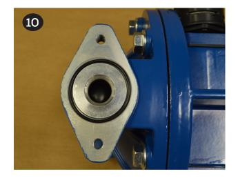
Check that the top of the seat (item 14) is about flush with the liquid chamber. Place the suction manifold (item 12) atop the pump. Tighten and torque the (4) suction manifold bolts (item11) in an "X" pattern.
