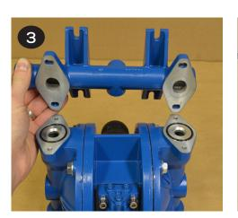
Remove both liquid chambers by removing the (6) bolts (items 16) on each liquid chamber using a 13mm (or ½") wrench. Inspect and replace diaphragms if needed.
