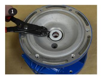
Use the supplied grease packets to lightly grease the OD and ID o-rings (items 23 & 26) that come preinstalled in the new shaft bushing (item 24) supplied in air end kits.
