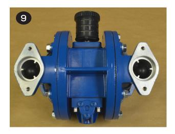
install (1) of the valve seat o-rings (item 13) into the liquid chamber (item 17) followed by the valve seat (item 14) and then another valve seat o-ring (item 13). The o-ring will fit into the groove created by the valve seat and liquid chamber.
