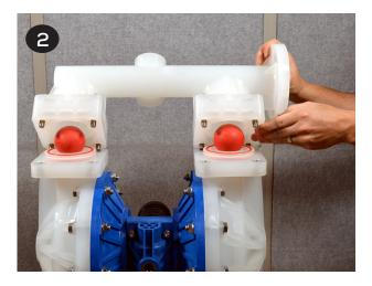
Repeat the above steps for the suction manifold (item14). The seat o-rings, valve seats and valve balls (items 15, 16, & 17) are located in the liquid chambers (item 20). Remove both liquid chambers by removing the (10) bolts, washers & nuts (items 18, 19 & 28) on each liquid chamber using a 17mm wrench and nuts can be removed using a 15mm wrench. Inspect and replace diaphragms if needed.
