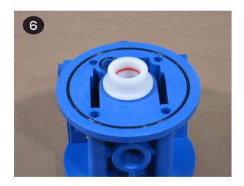
Install both air chambers (item 27) by placing one side on top of the center section (item 35). Ensure the air path hole of the center section lines up with the through hole in the air chamber. Insert the (4) bolts & washers (items 25 & 26) through the air chamber and center section. Flip the components over and place the remaining air chamber on the center section. Thread the nuts & washers onto the bolts (items 25, 26 & 38). Tighten and torque the fasteners.
