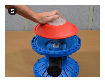
6 It may be easier to thread the molded in bolt into the shaft if the diaphragm(s) is inverted on one or both sides. This can be done by hand. The other diaphragm(s) (items 22/23) and inner/ outer plates (items 21 & 24) can be installed onto the opposite end of the shaft (item 32).
