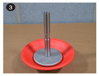
• The shaft (item 32) and shaft o-rings (item 31) should retain the lubricant that was factory applied. If they appear dry, apply a light coat of lithium thickened grease. Avoid over lubrication as it can cause decreased performance of the air distribution system.
