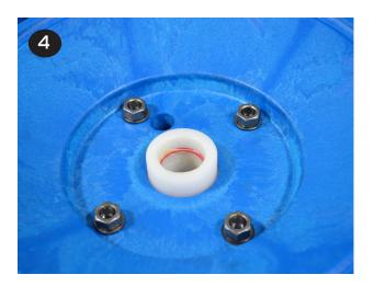
• Push the shaft (item 32) through the center of the shaft bushing (item 30). It is normal for this to be a tight fit, especially if the shaft and shaft o-rings (item 31) are in good condition.
