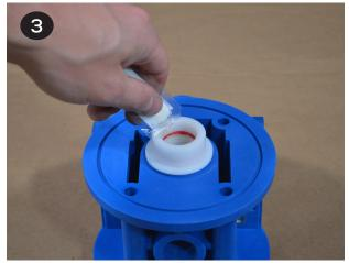
• Insert both bushings into the center section. Ensure the bushing is fully installed.
