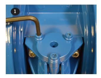
**C** Aluminum Air Valve - Remove and replace o-ring (item 8). Install cap (item 9), tighten, and torque the valve cap screws (item 11). Repeat for the remaining cap.
