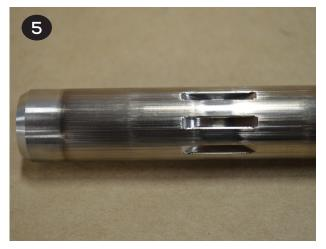
• After determining if the condition of the shaft is acceptable, ensure both center section o-rings (items 33 & 34) are in place on both sides of the center section.
