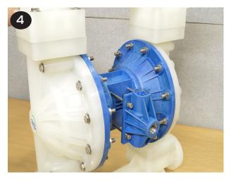
• Tighten and torque the (4) cap screws into the center section.
