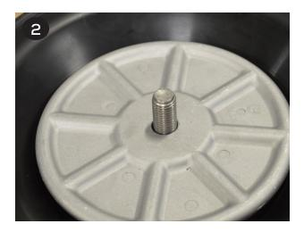
3 Apply a couple drops of a medium strength thread locker, such as Loctite® 246, to the molded in outer plate bolt (item 21). Thread the shaft (item 32) onto the molded in bolt until it is snug to the flat back side of the inner plate (item 24).
