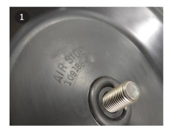
Place the inner plate (item 24) over the molded-in bolt. Ensure the round recess in the plate faces the diaphragm (item 23).
