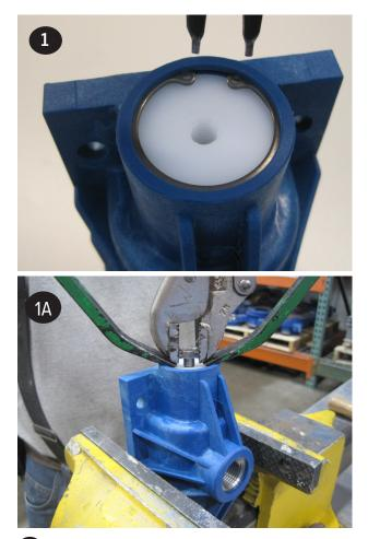
Plastic Air Valve - Remove and replace o-rings (item 8). Insert cap (item 9) and push down until groove for the retaining ring is visible. Install retaining ring (item 10). Make sure to lubricate the o-rings prior to inserting into the valve body with a compatible lubricant.
