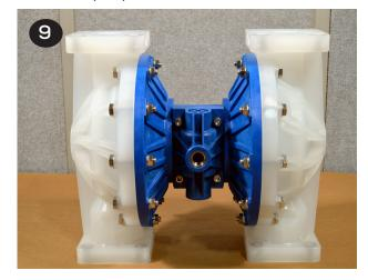
Flip the pump upside down and drop the suction valve balls (item 17) into the liquid chamber (item 20) ball cages.
