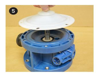
6 The other diaphragm(s) (items 20/21) and inner/outer plates (items 19 & 22) can be installed onto the opposite end of the shaft (item 27). It may be easier to thread the molded in bolt into the shaft if the diaphragm(s) is inverted on one or both sides. This can be done by hand.
