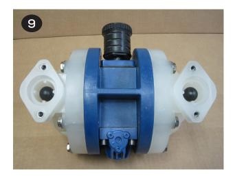
Place the larger valve seat o-rings (item 15) into the seat bores of the liquid chambers followed by the valve seats (item 14). Install the two smaller o-rings (item 13) into the face grooves in the valve seats. The seats are to be orientated so that the edge groove on the seat accepts the larger o-ring.
