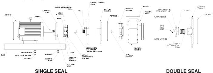
\* Shaft spacer (1 3/4" OD x 1/4" thick) to be used only with impellers that DO NOT have a metal impeller insert permanently attached to the impeller
