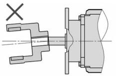
1-3 Press the magnet coupling in until the end of the motor shaft and the coupling (M) are at the same position.
