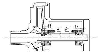
Clearance between Impeller and casing
