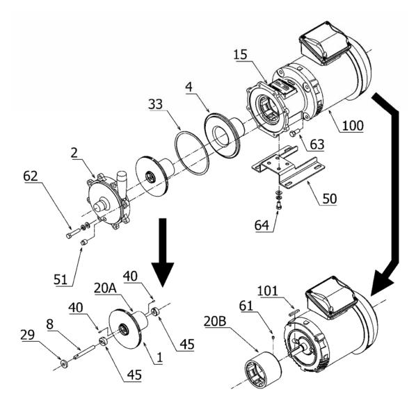
• When the liquid being handled is a hazardous chemical, drain the liquid and then clean the pump thoroughly before disassembly. Small quantities of liquid will remain on the threads, spigot joint sections, and interface sections inside the pump. Therefore, when handling chemicals that are hazardous to human health, be sure to wear protective gear (safety goggles, rubber gloves, etc.) and be very careful during disassembly.
