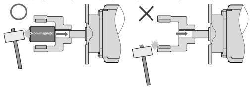
1-2 Press the magnet coupling straight onto the motor shaft. If it is at an angle, the shaft may be damaged.
