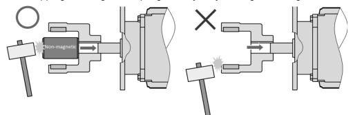
1-2 Press the magnet coupling straight onto the motor shaft. If it is at an angle, the shaft may be damaged.
