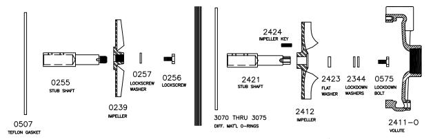
NEED TO BUY IMPELLER, STUB SHAFT, KEY, LOCKDOWN BOLTS/WASHERS, O-RING AND VOLUTE
