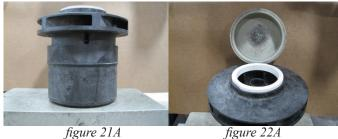
5. Impeller can now be reinstalled back into the pump. Feel free to contact Finish Thompson, Inc if you have questions @ 1-800-888-3743.
