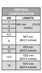
HORIZONTAL CONFIGURATION kW LENGTH 2 508 mm (20 inches) 3 4.5 629 mm 6 (843.5 inches) 845 mm (843.5 inches) 9 12 13.5 1066 mm (843.5 inches) 18
